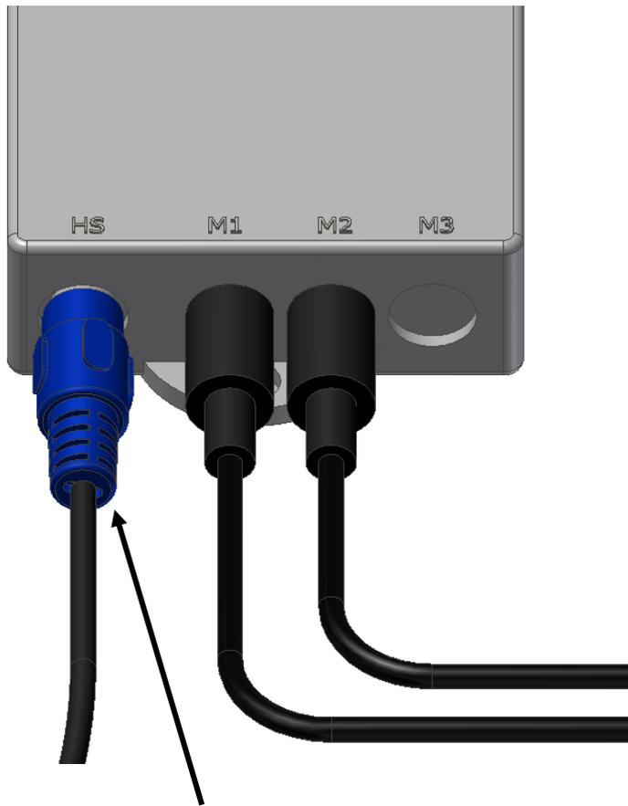
Connect the receiver to HS input
