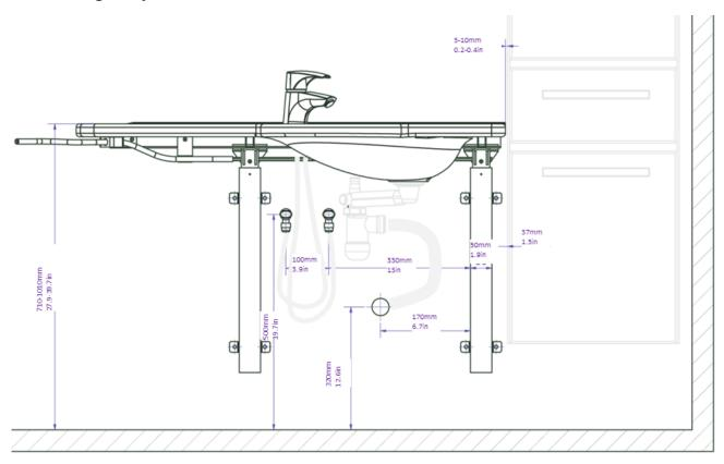
We recommend positioning of water and drain installations as illustrated. It is important that all hoses for water and drain installations are flexible to ensure unhindered movement of the frame within the height adjustment range from 71-101 cm/28 – 39.8in (including washbasin).
