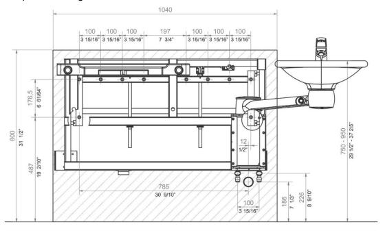
**NOTE:** All dimensions are based on adjustment of the washbasin from 750 - 950 mm (29  $\frac{1}{2}$ " – 37  $\frac{2}{5}$ ") above floor level. If a change of this height-adjustment range is required, the recommended dimensions must be changed accordingly.
