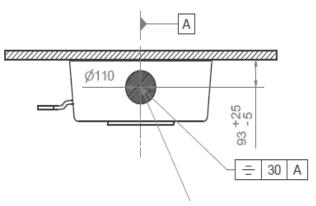
Floor drain must sit flush with floor
