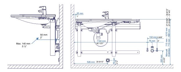
Manual/Electrical height adjustment, plumbing visible beside the washbasin. (plumbing may be located on either side of the washbasin).
