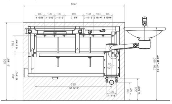
**NOTE:**All dimensions are based on adjustment of the washbasin from 750 - 950 mm ( $29 \frac{1}{2}$ " – 37 2/5") above floor level. If a change of this height-adjustment range is required, the recommended dimensions must be changed accordingly.
