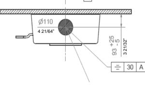
Floor drain must sit flush with floor
