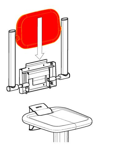
Please note: Mount only the PUR backrest under tempered conditions. At 10  $\,\mathrm{C}^\circ$  or lower the backrest surface could crack during mounting.
