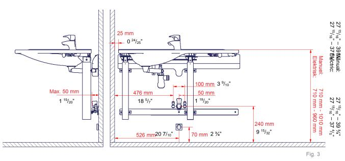
All hoses for water connection and drain must be flexible for the washbasin to move freely within the range of adjustment.
