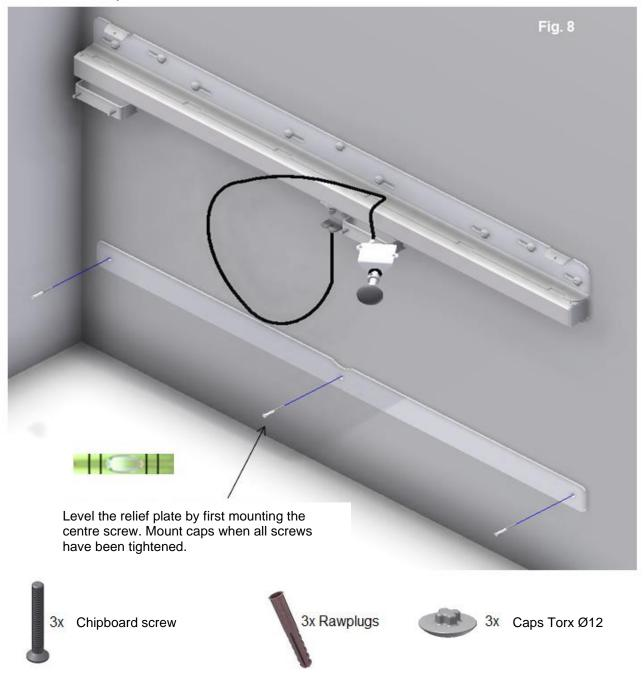
Mount the plastic cover in the screw holes of the wall rail
