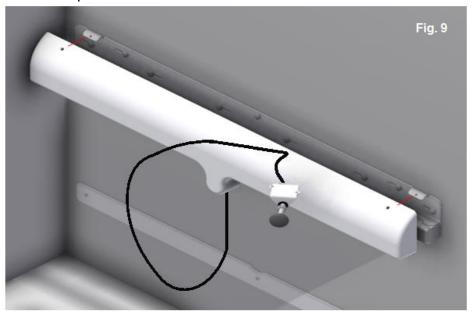
Fasten the plastic cover and press the caps onto the screws.
