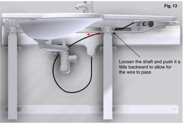
Place the wire behind the frame ensuring free movement
