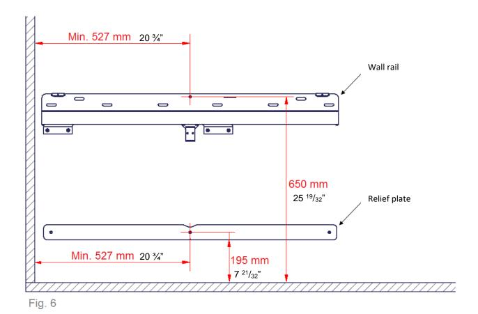
The marking shown has been made so as to avoid jamming between the washbasin and the adjoining wall. The minimum distance of  $527mm / 20 \, \%$  is decisive for avoiding the risk of jamming.
