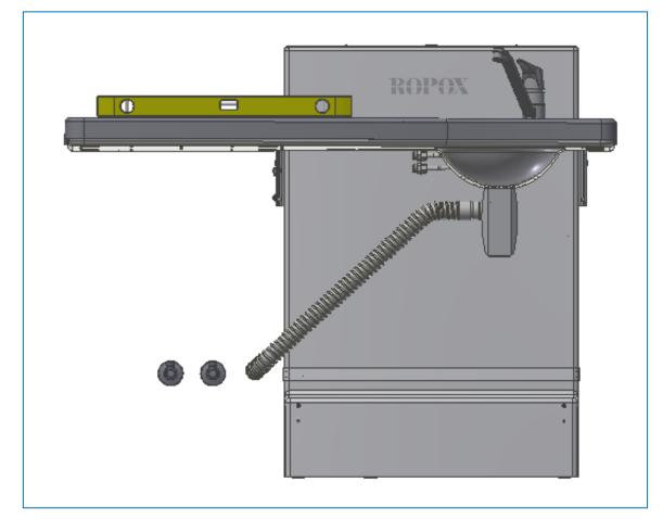
6. The nursing table is now installed. If the tabletop unit is still not level, it's possible to adjust it. This is done by tightening/loosening the screws in the sides.
