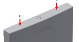
3. The tabletop unit can now be mounted on the lifting unit. The tabletop unit comes pre-assembled.
