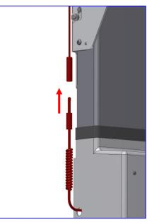
5. The water and drain can now be mounted. Drain hoses and water hoses come with the product.
