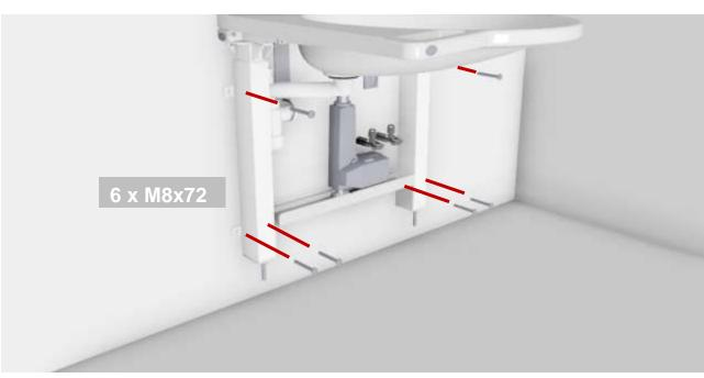
NOTE: Depending wall type, choose other suitable screws, as required. Max. load on upper screws: 71 kg / 156 lb /screw
