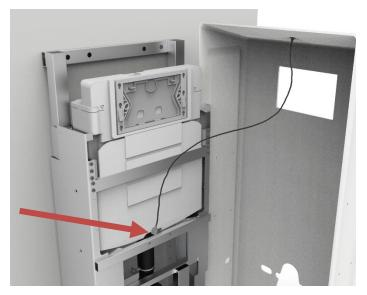
**D.** Guide the cable along the front of the lifting unit and pull it <u>behind</u> the cross bar below the cistern, as indicated on the illustration.
