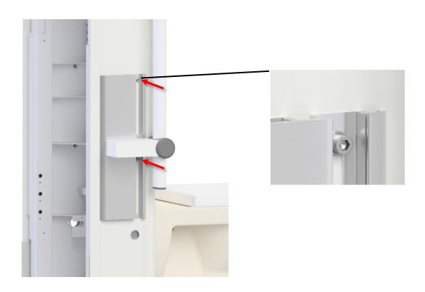
**d.** Test the toilet support arms in the horizontal direction. If they can twist significantly, dismount the assembly and leave <5mm between the underside of the screw head to the plastic cover. There should be no clearance between the aluminum bracket and plastic cover. Adjust until the support arms are properly fastened.
